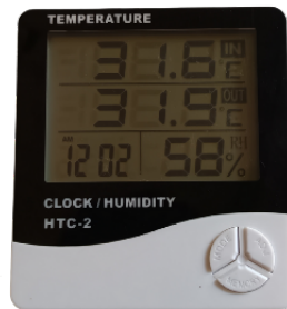
Gambar 2. Termometer Digital ( thermo-hygrometer )
