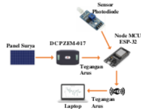
Gambar 4. Diagram Sistem Monitoring STSA
