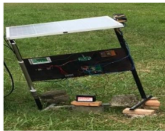
Gambar 2. Konstruksi Solar Tracker Single Axis
