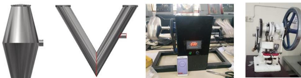
Gambar 2. Tabung mixer *double cone*, V-25°, mesin mixer ganda 2D, mesin cetak tablet
