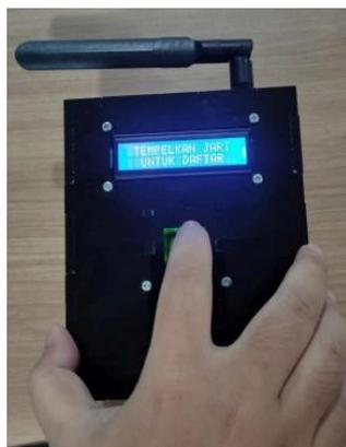
Gambar 3. Alat Fingerprint
