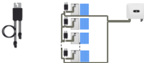
Gambar 1. Skema Smart PV Optimizer
