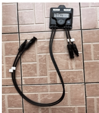
Gambar 5. Alat Smart PV Optimizer
