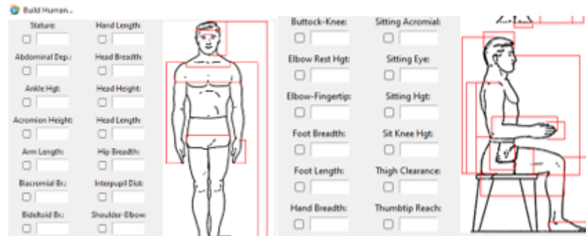
Gambar 2. Dimensi Antropometri Berdasarkan Software Jack Sumber: Software Technomatic Jack 8.4
