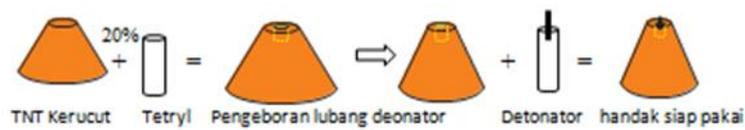
Gambar 6. Model Kerucut
