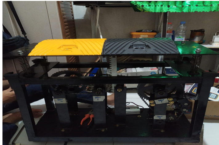
Gambar 1. Road Power Generator
