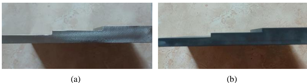
Gambar 1. Spesimen hasil proses Milling. (a) Material SS 304. (b) Material PVC
