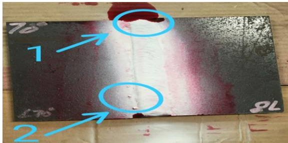
Gambar 21:: Cacat Las Undercut (1), Over Spatter (2)
