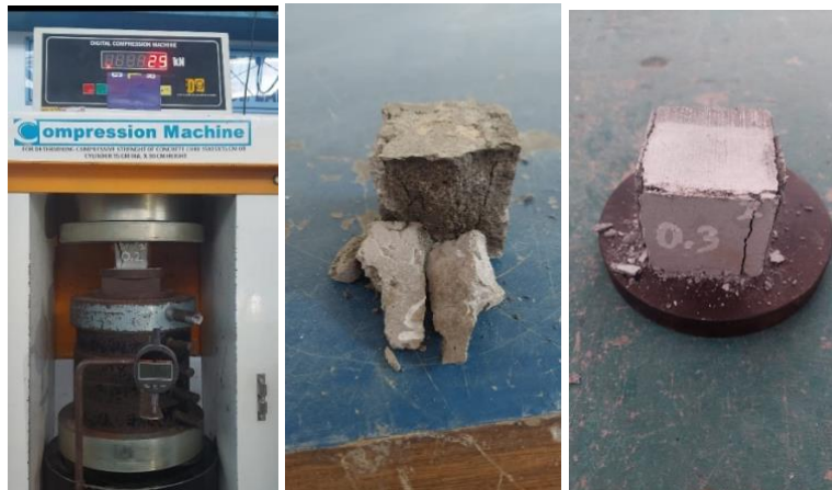
Figure 5. Compressive strength testing and final results of mortar samples
