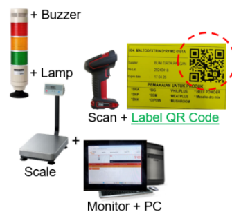
Figure 2. QR Code System to Prevent Recipe or Material Errors
