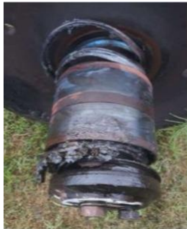
Figure 2. Failure in railway bearing
