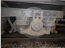
Figure 1. Tapered Roller Bearing in railway vehicle
