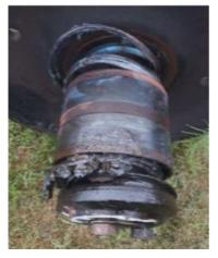
Figure 2. Failure in railway bearing
