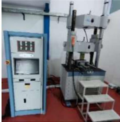
**Gambar 2.** Mesin Uji kalibrasi Micro Computer Servo Hydraulic Universal Testing Machine (100 Ton)
