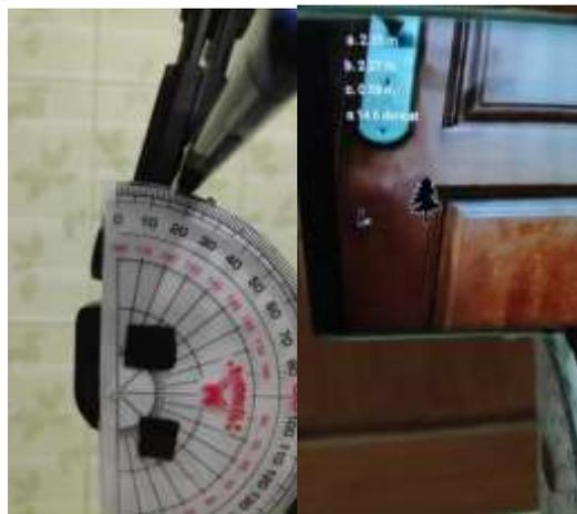
Gambar 4. Proses kalibrasi sensor gyroscope smartphone
