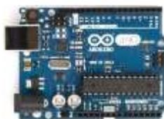
Gambar 1. Arduino UNO R3 ATmega328
