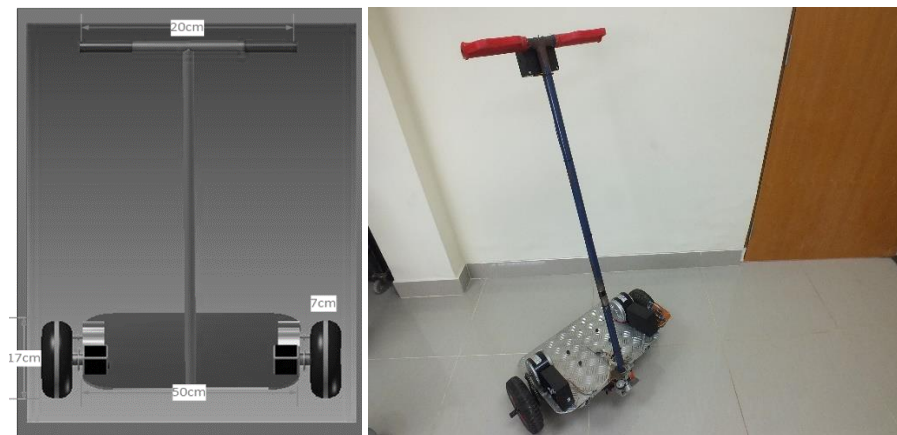
Gambar 4. Desain Mekanik Self-balancing Two Wheel Electric Vehicle (Scooter)
