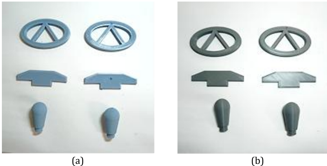
Figure 4. The printing results of each object from a) Ender 3 Pro, b) Anycubic Photon 3D printing machine
