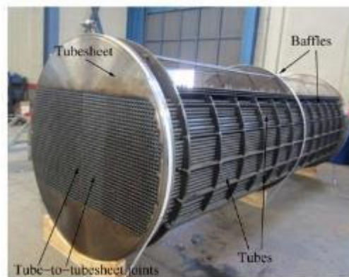
Figure 1. Tube to Tubesheet on Heat Exchanger [2]
