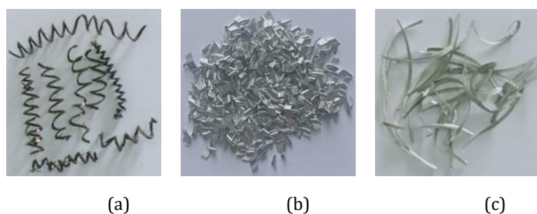
Figure 7. The potential differences in the chip morphology obtained in; (a) turning, (b) milling, and (c) turn-milling
