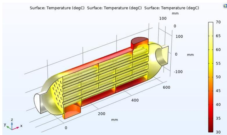
Figure 5. Temperature profile on the heat exchanger surface
