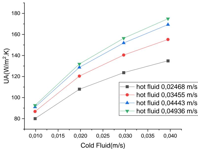
**Figure 3.** Graph of Velocity Effect on UA
