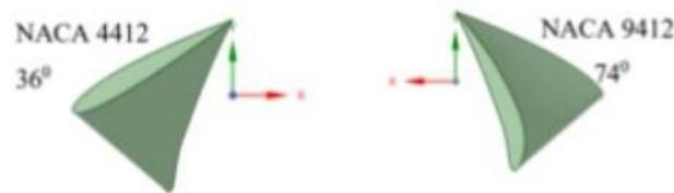
**Figure 8** Airfoil type and blade angle of attack
