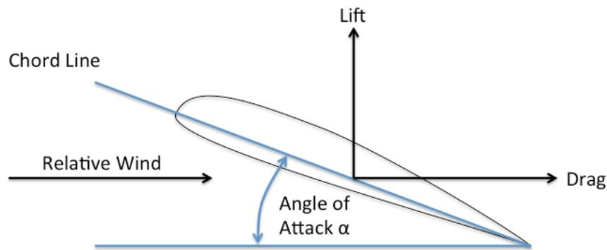
**Figure 2** Angle of attack cause lift [4]
