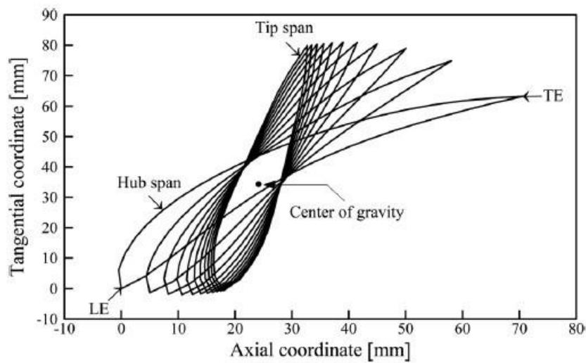
**Figure 5** Shape of the airfoil based on altitude [8]
