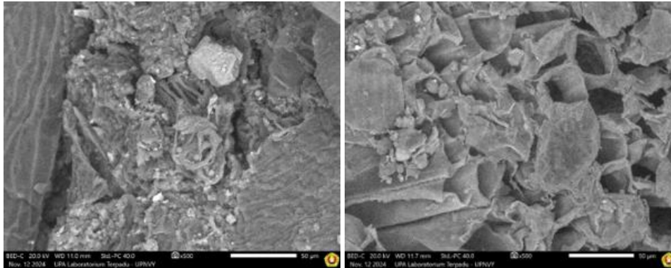
Figure 4. Biomass Surface Morphology Before (left) and After (right) 500 x Magnification
