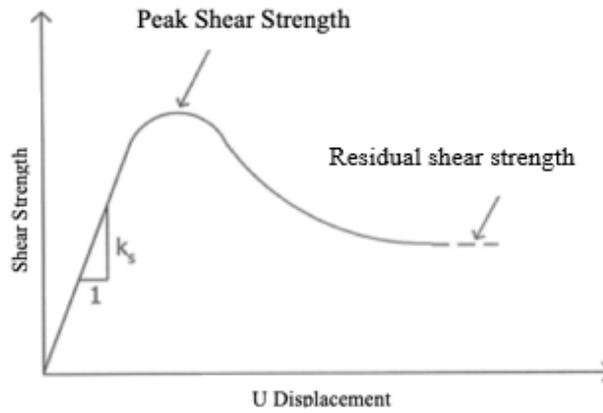
**Figure 3.** The stress yield curve and shear displacement with constant normal stress values [31]
