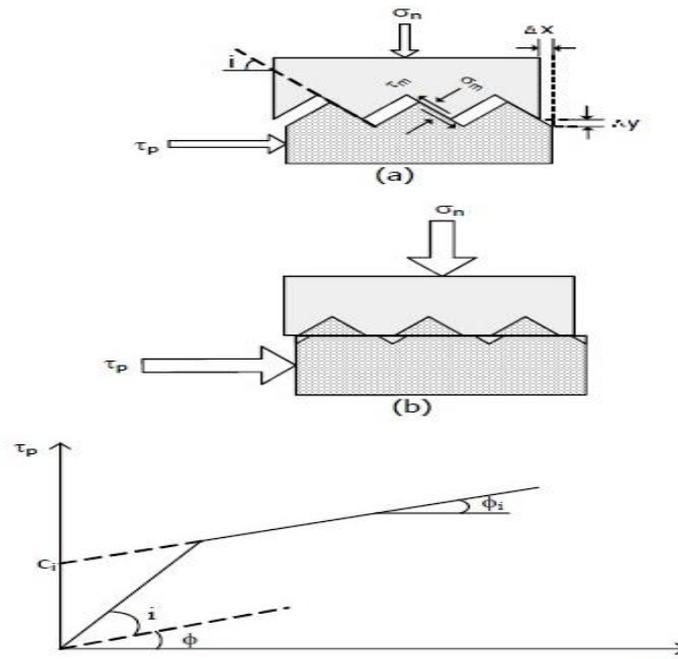
**Figure 5.** Shear roughness, (a) and (b) failure mechanism, (c) strength sheath [27]
