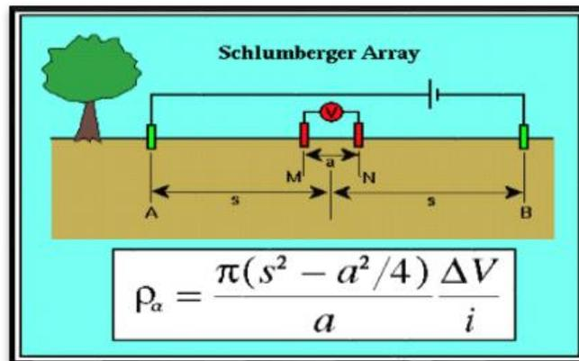
**Figure 1.** The schematic electrode on Schlumberger Configuration [1].
