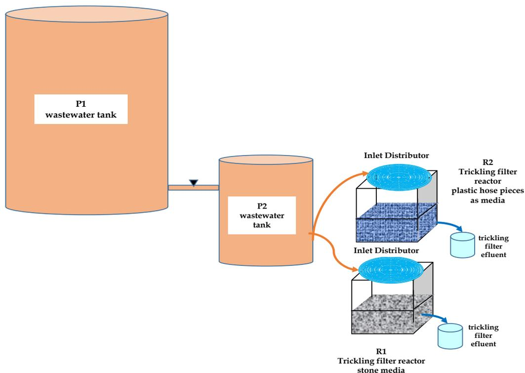
Figure 1. Experimental reactor setup
