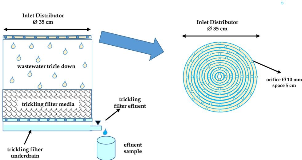
Figure 2. Detailed Tricking Filter Reactor Experiment
