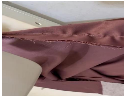
Figure 2 Puckered Seam Uniform Clothing
