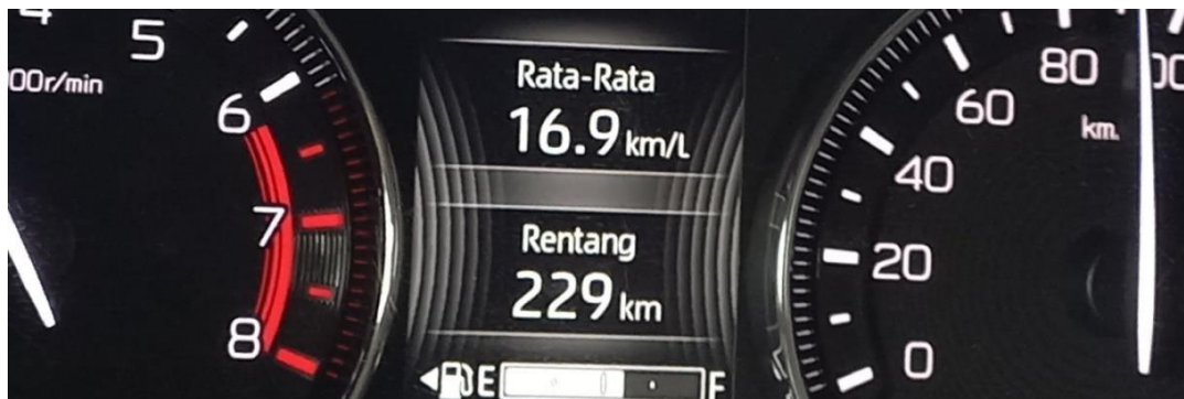
Figure 6. Example of MID display result of Highway Test.
