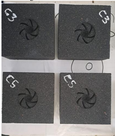
Figure 22. Chromite – chamotte sand mold before Shaw and Unicast processes.
