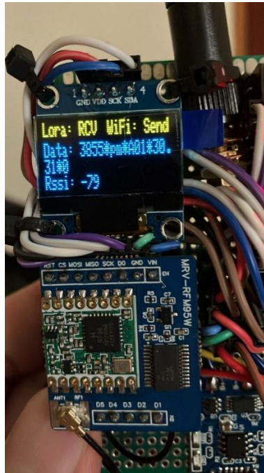
Figure 2. IoT Predictive Maintenance Microcontroller
