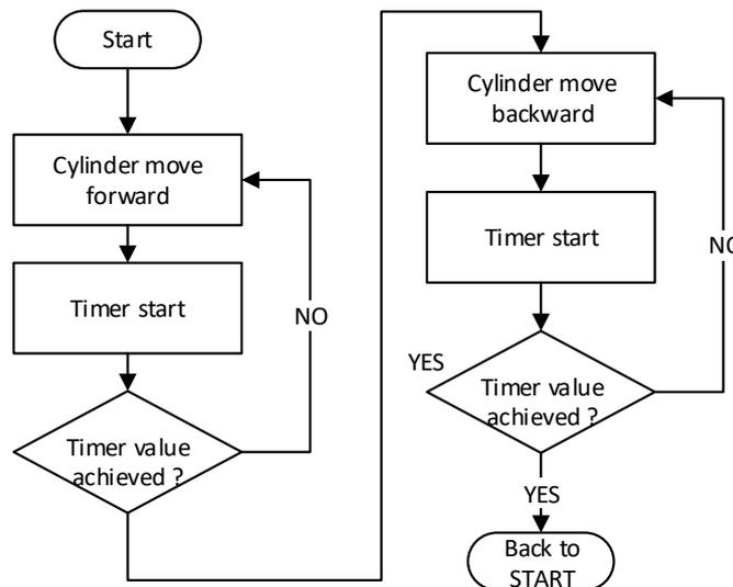
Figure 3. Cylinder moving sequence chart.
