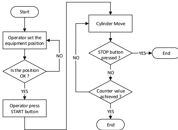
Figure 2. Simple process sequence chart.
