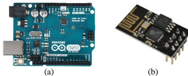
Gambar 3 (a) Arduino uno, (b) NodeMCU ESP8266
