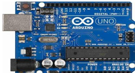
Gambar 1. Modul Arduino Uno
