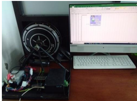
Gambar 7. Hardware Monitoring Perubahan Tegangan Motor BLDC
